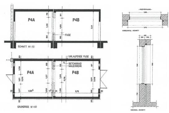
The maximum weighted sound reduction index of the test facility is R'w,max = 72 dB (related to the test opening area).
