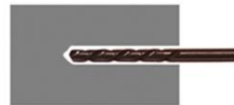
1. Pre-drilling of a hole and clean up the hole
