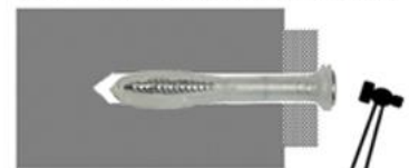
3. Hit the screw anchor with a hammer. Insert it into the screw anchor plug and tightened with an electric drill
