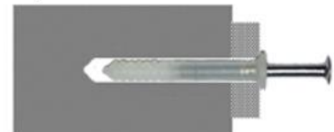
2. Push the product on the wall tightly and insert the screw anchor
